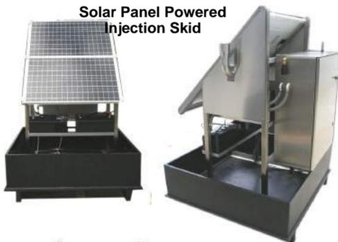
Solar Panel Powered Injection Skid
