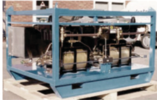
HIGH PRESSURE, HIGH FLOW, GLYCOL INJECTION SKID
