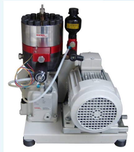
Compressor group equipped with electric motor and V-belt drive
