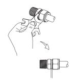
If the gauge can not enter the gap, the fitting is sufficiently tightened.
